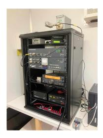
Above: Equipment arrangement, August 2023. The homebrew transmitter in the centre of the rack contains the Zachtek WSPR exciter and two power amplifiers (one each for LF and MF). The main station multi-mode exciter and receiver is a Kenwood TS-590S transceiver, on the shelf above the power supplies. To the right of the rack is the hand-held remote variometer tuning control.
