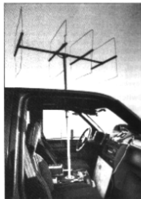
Fig 23.100 — K80V uses this mobile setup for RDF on several bands, with separate antennas for each band that mate with a common lower mast section, pointer and 360° indicator. Antenna shown is a heavy gauge wire quad for 2 m.
